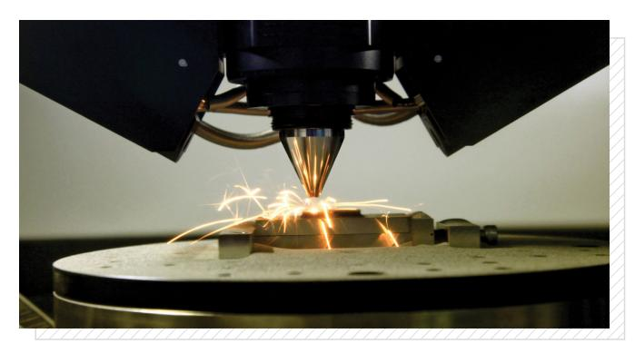
Additive manufacturing (AM), or 3D printing, refers to multiple manufacturing processes that build parts by adding material layer-by-layer, thereby replacing or augmenting more traditional manufacturing processes such as casting and forging. AM can shrink the supply chain and lead times for specialized and complex parts, introducing new efficiencies driven by design innovation, reduced manufacturing time, and improvements in part availability.
