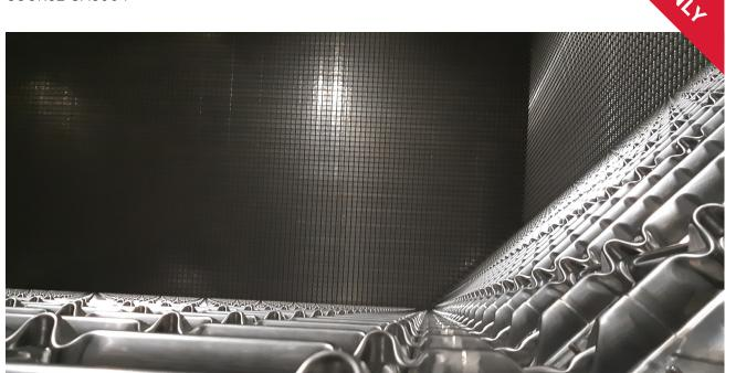
What's the difference between gas cargo containment systems? This course provides an overview of containment systems for safely transporting liquefied gases in bulk, including characteristics, support systems, materials and insulation, and advantages and disadvantages of the different types.
