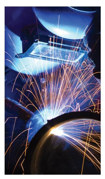
A good-looking weld surface appearance is typically considered of high weld quality. However, surface appearance alone does not equal good workmanship or internal quality.
