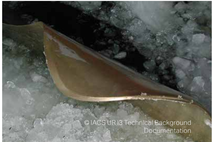
Damaged propeller blade from ice impact
