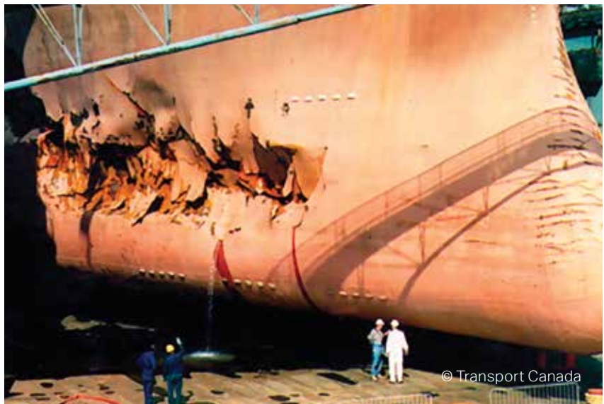
Damage from iceberg impact
