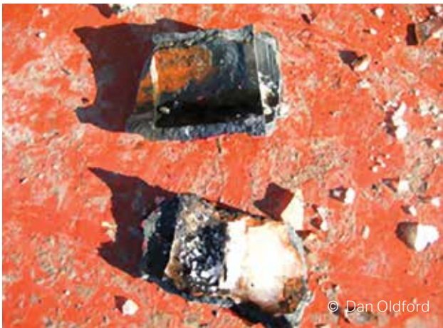
Material failure due to freezing and expansion of non-drained fire main
