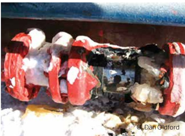
Material failure due to freezing and expansion of non-drained fire main
