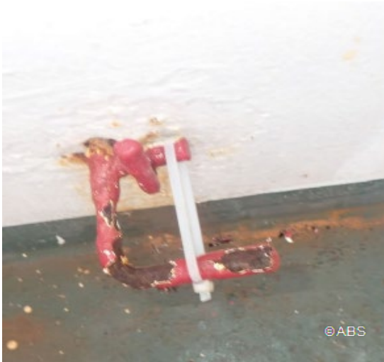
Man Overboard Buoy (MOB) unable to release due to operating mechanism stuck caused by wasted release handle
