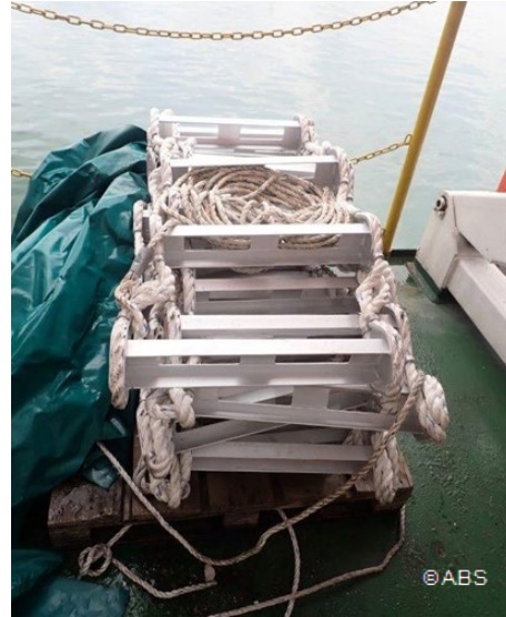
Non-compliant pilot ladder, i.e., no rubber steps, loose chocks and retrieving lines not secured as required
