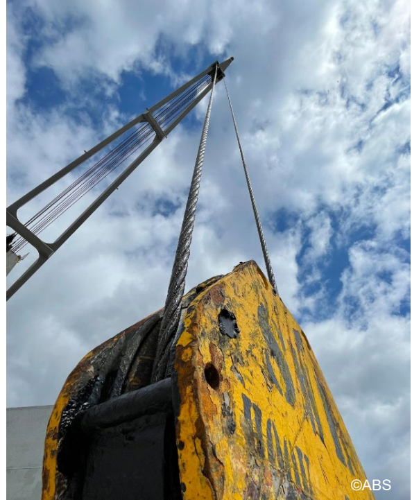
Cargo crane wire renewed – after
