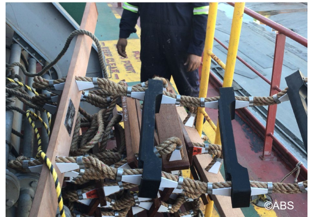
New pilot ladder provided
